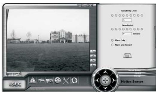
In this mode of automatic recording the software detects changes in the selected image to detect movement. When motion is detected an alarmsound can be given from the PC and a recording can be triggered.
